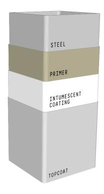
Fontefire ST 60-1 intumescent coating, together with an approved Tikkurila primer and topcoat, provides a complete system for fire protection.
